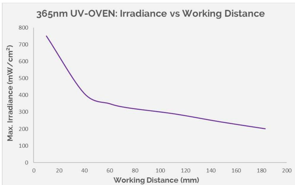
Curve plotted for UVA wavelength. Radiometer: GIGA HERTZ OPTIK RCH-116 (June 2023).
